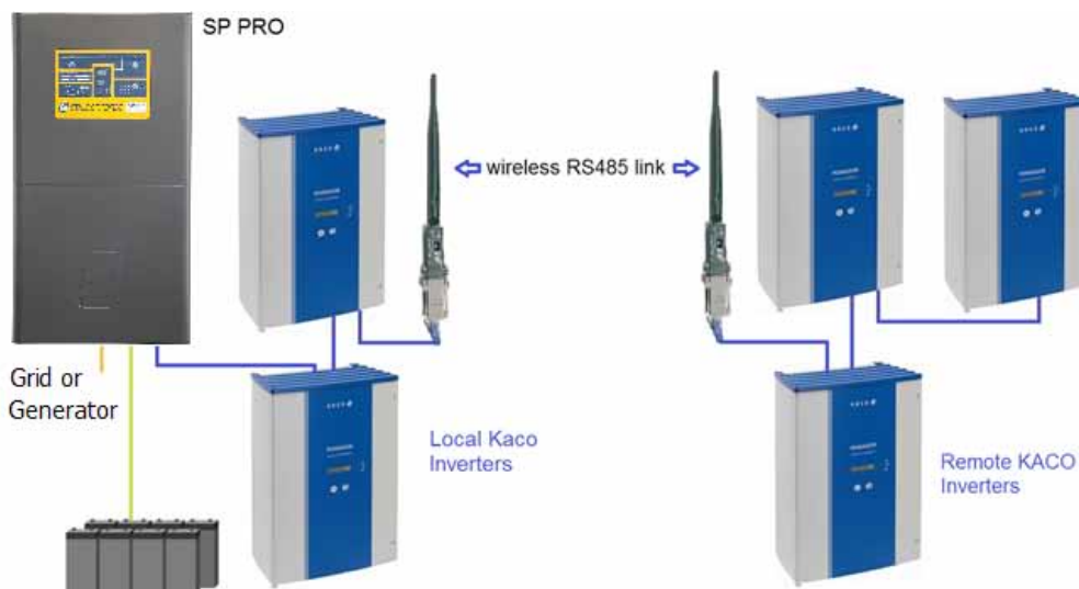
RS485 wired AND wireless communications links between SP PRO and KACO inverters
